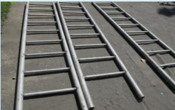
PETRON CORPORATION Fabrication of Stainless Steel Ladder and 8"Ø Pipe for the Repair of Pier and 8"Ø Riser Pipe
