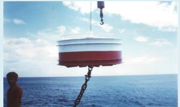
Completed unit of Mooring Buoy with Chain Attachment
